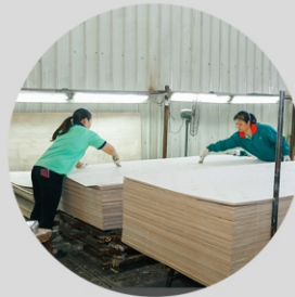
patching of base plywood
