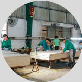
patching of veneered plywood
